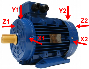
Figure 11: Measuring Points on Electric Motors
