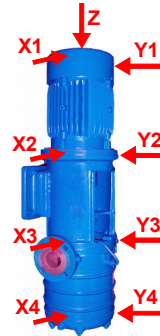
Figure 12: Measuring Points on Machines with Vertical Rotors
