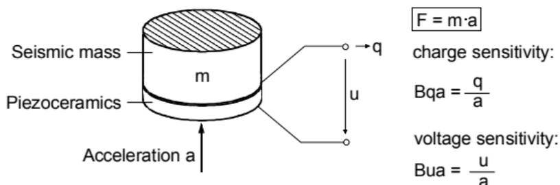
Figure 2: Principle of a piezoelectric accelerometer
