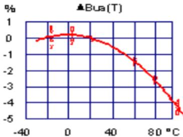
Figure 9: Example of non-linear temperature / sensitivity curve
