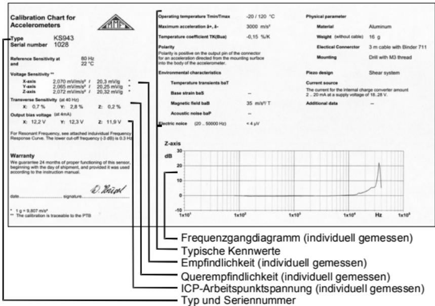
Figure 8: Individual calibration chart of Metra accelerometers
