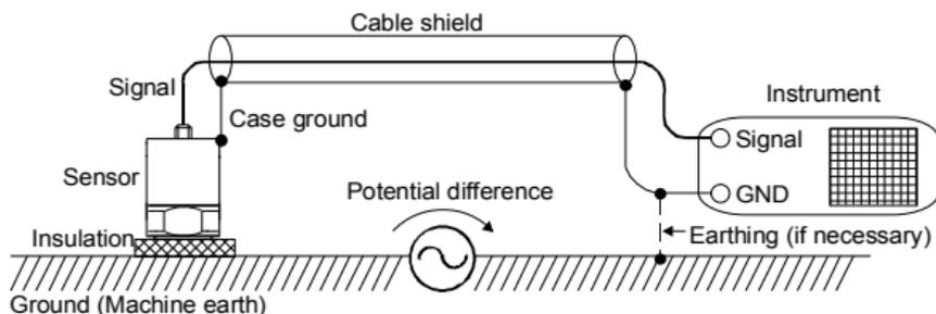
Figure 23: Insulated sensor mounting avoids ground loops
