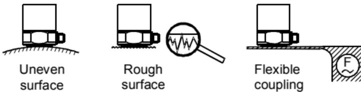
Figure 17: Typical reasons of coupling errors
