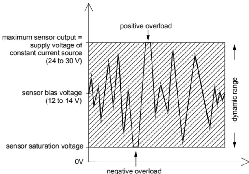
Figure 14: Dynamic range of IEPE compatible transducers
