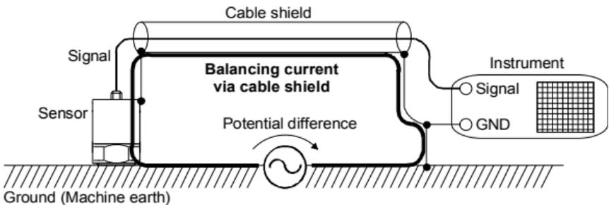
Figure 22: Sensor mounting without insulation causes ground loop
