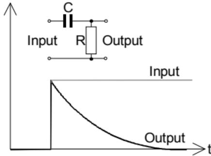
Figure 15: Step response of IEPE transducers
