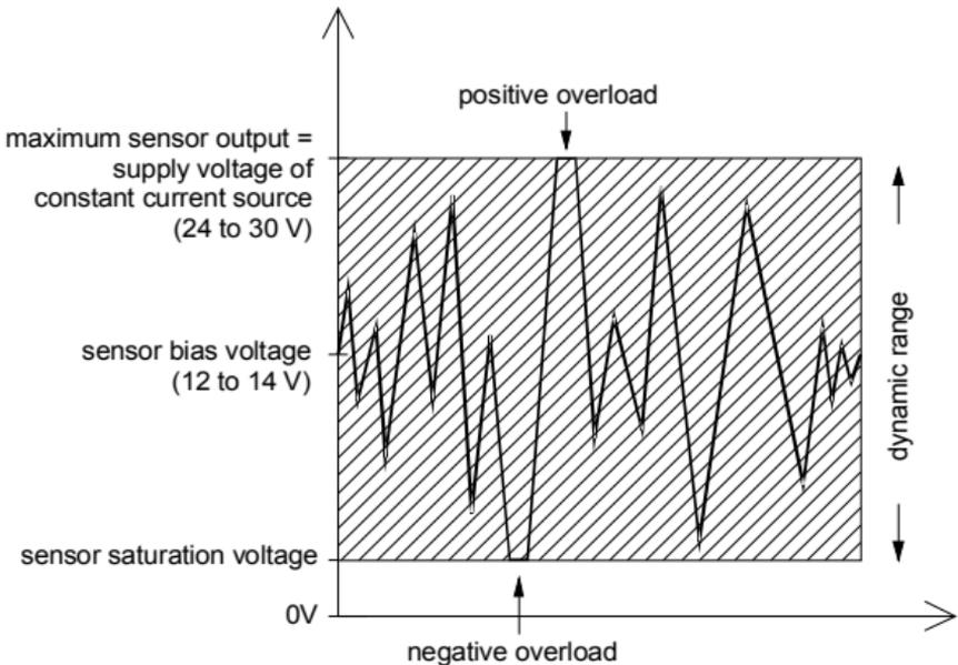
Figure 5: Dynamic range of IEPE compatible transducers
