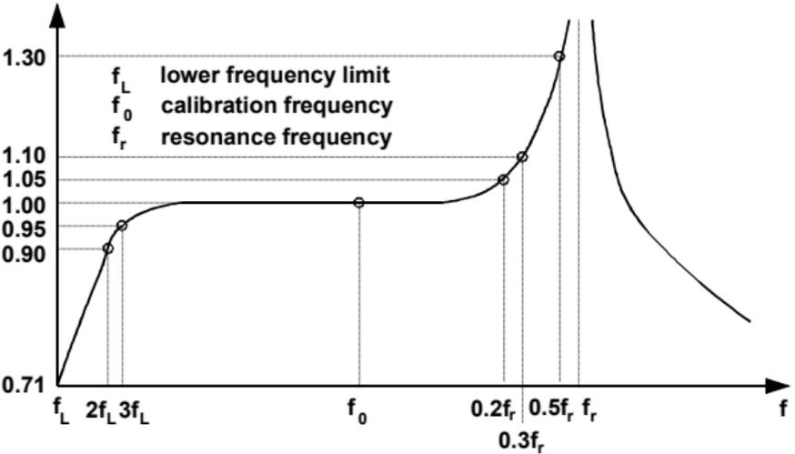
Figure 3: Frequency response curve
