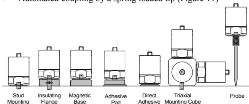
Figure 18: Mounting methods for accelerometers
