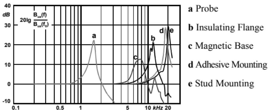
Figure 20: Resonance frequencies of different mounting methods
