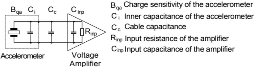
Figure 12: Charge accelerometer at high impedance voltage input
