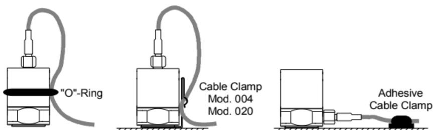
Figure 21: Methods of cable tie-down
