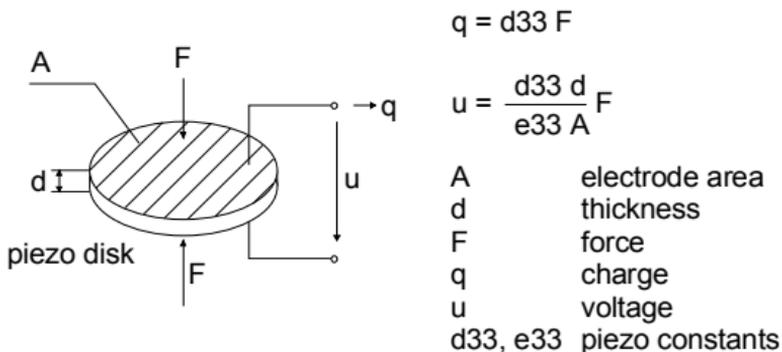
Figure 1: Piezoelectric effect, basic calculations
