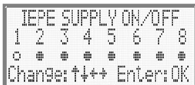
Figure 17: Switching the IEPE supply on or off
