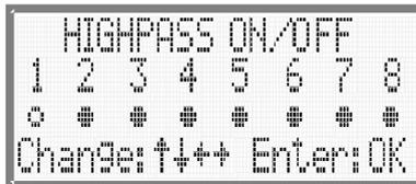
Figure 16: Switching high pass filters on or off
