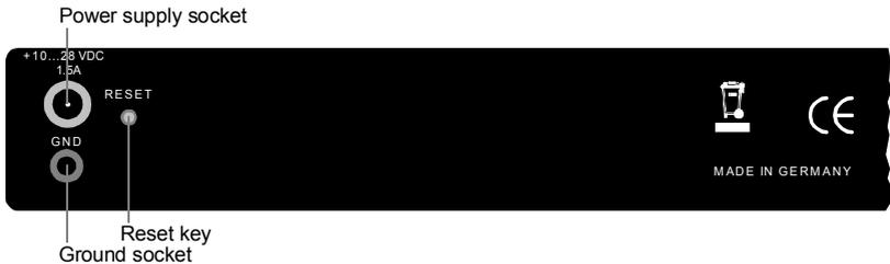
Figure 1: Front and rear panels
