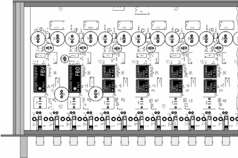
Figure 15: Location of the filter and integrator modules
