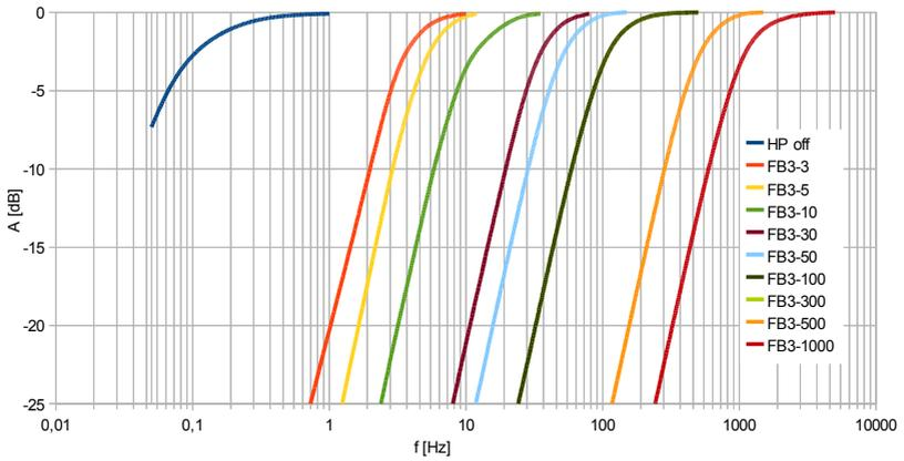
Figure 9: Frequency response of M208B with different high pass filters FB3-...
